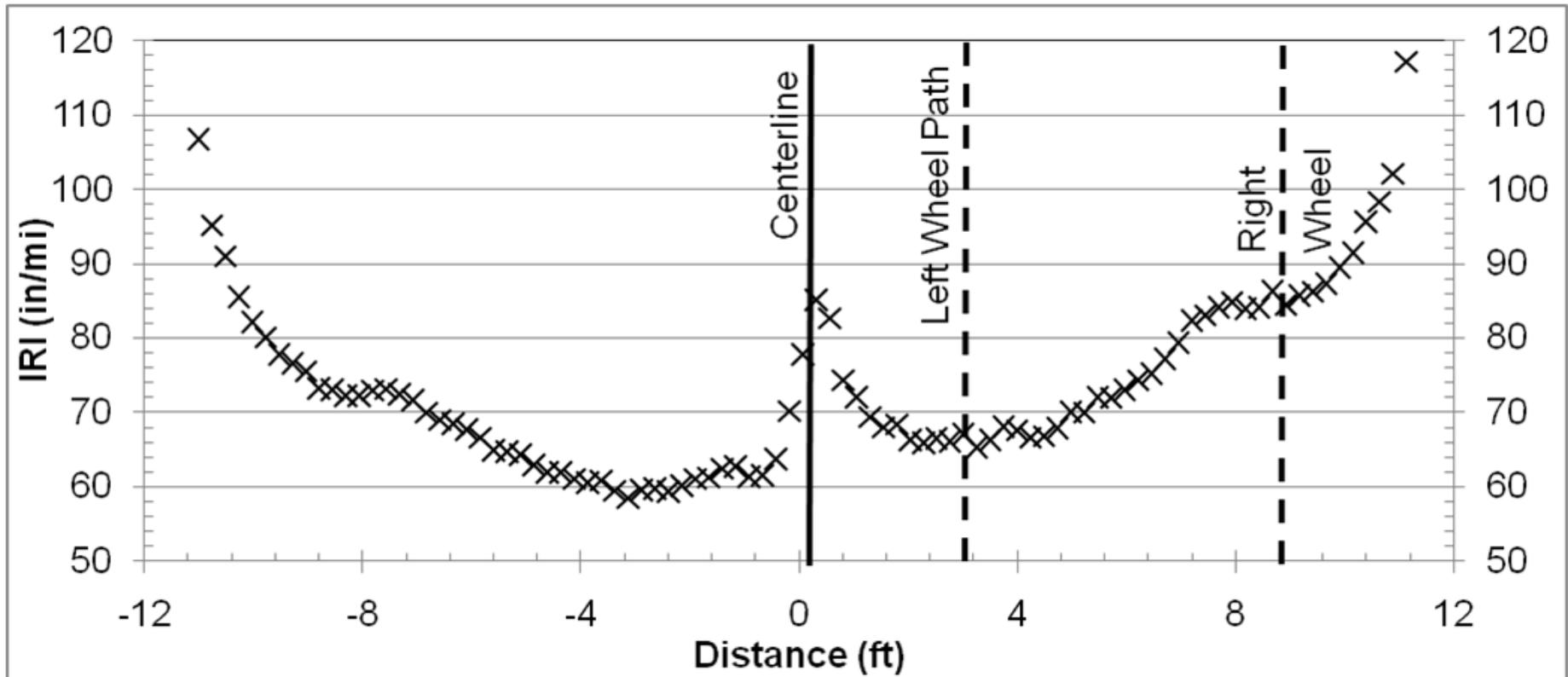
IRI determined across the roadway for profiles spaced every 3" using a 3" point spacing
